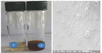
Change of colour in solution and SEM images of silver nanoparticles
