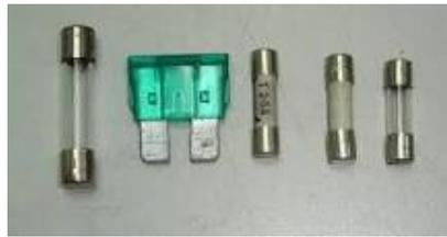
It is strongly recommended that fuse wires of correct current rating should be used. **DO NOT INCREASE THE FUSE CAPACITY FOR PREVENTING OR ELIMINATING FREQUENT FUSE BLOW-UPS.** It is essential to locate the causes and eliminate the same. Replacing fuse wires of higher capacity may invite troubles in the form of fire & damage to supply system and surroundings.
