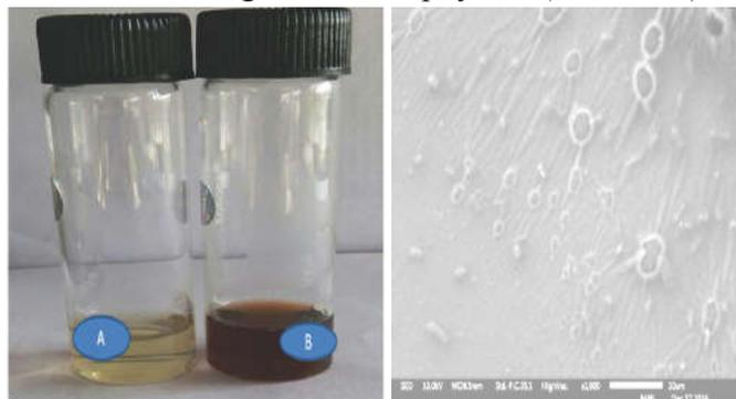
Change of colour in solution and SEM images of silver nanoparticles
